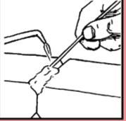
4. With joint surfaces thoroughly tinned, flow in enough rod to fill the vee. Be sure filler metal fuses with the tinned surface without melting the base metal.
