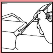
Heat welding rod to same temperature. With both the base metal and rod at this temperature, touch the rod to the break. It will flow into the vee, fusing thoroughly.
