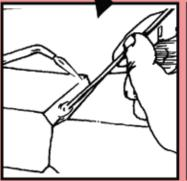
2. Heat the metal hot enough to flow the rod without the aid of the flame, thoroughly tinning the surface.
