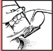
3. Turn and tin the beveled surface, building new metal until slightly larger than its original size. Remove temporary support with minimal heat.
