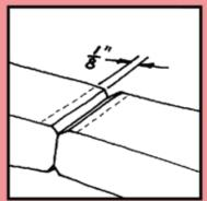
1. Vee the broken edges of the area to be repaired to about 45°. Clean the surface of any plating or scale back from the edges of the vee 1/8 of an inch.
