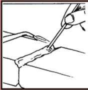
4. Continue until break is completely filled. Be sure to kick rod into weld to break down skin resistance or filler rod will lav on the surface and will not fuse.
