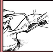
2. Heat metal hot enough to flow rod without the aid of the flame. Tin the flat side of the blade and attach a piece of carbon or copper to support the repair temporarily.
