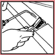
Brush surface to be repaired thoroughly under heat to break up surface oxide.
