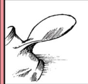
Let the repair cool, then grind to proper pitch standards. You now have a complete repair without porosity ready to balance and paint.
