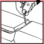
Heat metal until it starts to flow. Turn flame parallel to surface, and hold metal at this heat with the indirect flame.
