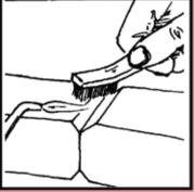
Brush tinned surface under heat, thoroughly filling the open pores.
